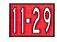
DETAIL "B" TYPICAL MANDATORY RUNWAY HOLD POSITION SIGN. SHALL CONFORM TO FAA AC 150/5340-18, MOST RECENT EDITION. NTS
